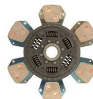
Lamela spojky priemer 310 mm, DEUTZ FAHR, LAMBORGHINI, MASSEY FERGUSON, SAME
